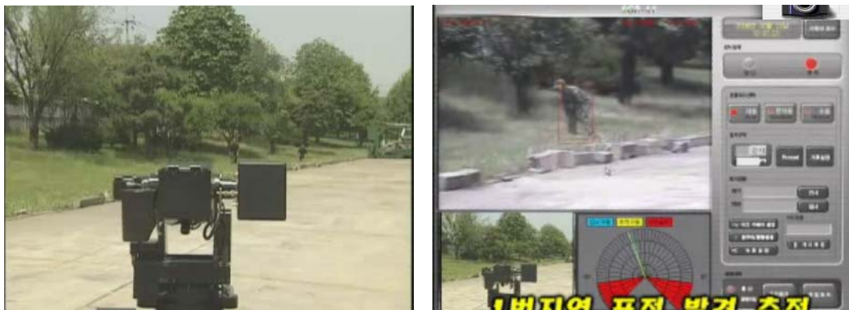
Figure 22: (Left) Samsung robot in a test scenario (Right) The operator display. Note the target identified by a bounding box.
